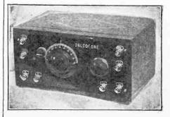
Trade Name — "Dalcofone"; Type — Radio Frequency; Battery—"A" Storage or Dry; "B" 90 Volts; Tube--1; Controls—Tuning, 1; Tube, 1; Antenna—Outdoor; Dim.—11½ x 5½ x 7; Wt.—3 lbs.; Price—\$8.75.
