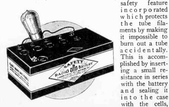
this resistance being of such dimensions that it does not in the least interfere with the normal operation of the battery in supplying the minute currents required for the plate circuits, and yet limiting the current which could flow in case of short circuit to less than required to damage a filament.
