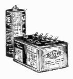
Trade Name-"Re-Vi-Vo"; Types-"A" and "B" (rechargeable dry cells); Capacity-"A" 15 A.H., 1.6 volts; "B" 1½ A.H., 22½ volts and 45 volts; Material of Case-Zinc; Price-\$0.50, "A"; \$2.00 and \$4.00, "B".
