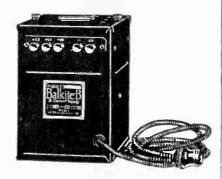
Trade Name-"Balkite B"; Type-Electrolytic; operates from 110-120 volts, 60 cycles, A.C.; also made for 50 cycles; delivers current of 40 milliamperes at 90 volts, with taps for varying output to meet requirements of various sets; replaces "B" battery; Material of Case-Terne plate, enameled; Dim.-71/4 x 6 x 9 in. high; Weight-10 lbs.; Price-\$55.00.
