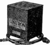
Model 00 Trade Name-"Unitron"; Type-Bulb; operates from 110 or 220 volts, A.C., 25, 40 or 60 cycle; Charging Rate-2½ amperes; attachment for charging "B" batteries; Material of Case-Metal; Dim.-6¼ x 6¼ x 8½ inches high; Weight-9½ lbs.; Price-\$18.00.
