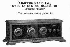
Model De Luxe Trade Name — "Deresnadyne"; Type — Non-oscillating Radio Frequency; Tubes—5; Battery — "A" Storage; "B" 90 Volts; Controls—Tun-ing, S; Tube, 3: Dim.—27½ x 9¼ x 9; Wt.— 80 lbs.; Price-\$165.00.
