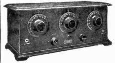
Trade Name — "Masterpiece"; Type — Tanes Radio Frequency; Tubes — 5; Battery — "A" Stanage or Dry; "B" 90 Volts; Controls — Tuning, 3; Tube, 2; Dim. — 7 x 7 x 18; Wt. — 21 Wos.; Price — \$60.00.
