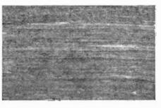
work, can be drilled, sawed, threaded, engraved or stamped without chipping or cracking. It will take a wood screw without drilling. Its surface is glossy and has the general appearance of highly polished hard wood. It is furnished in black, red and brown mahogany.
