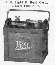
Model DXA Trade Name--"USL"; Type--"A"; Capacity--Made in 6 sizes, 30-140 A.H.; Material of Case --Hard rubber; equipped with bushing cover, rubber gaskets, aluminum wing nuts and nickelplated bail handle; Finish-Black; Dim.-----; Price--\$6.20, \$7.60, \$14.70, \$18.90, \$24.00, \$30.05.
