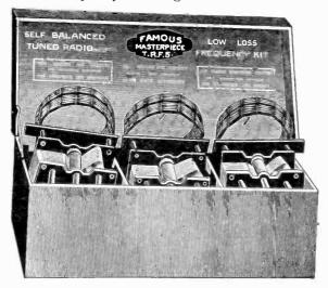
prises three micrometric brass condensers and three tuned radio frequency coils, with a complete diagram and step-by-step instructions for building the set. It is claimed that the resulting set will be self-balanced, nonoscillating, and that no neutralizing condensers are required.
