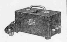
Trade Name—"B-Radicator"; Type—Bulb rectifier with filter circuit, 1 or 2 bulbs, rectifying both sides of wave with 2; replaces "B" battery. Dim.— $10 \times 4\frac{1}{2} \times 6$  in.; Weight—13lbs.; Price—\$45.00 without tubes.
