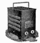
Trade Name-"Electron Junior"; Type-Bulb; operates from 110 volts, 60, 50, 40 and 25 cycles, A.C.; Charging Rate-2 to 8 amperes, 6 or 12 volts; Material of Case-Sheet metal, enameled; Weight-11 lbs.; Price-\$18,60.
