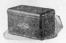
Trade Name—"Run-a-Radio"; Type—Bulb rectifler with filter circuit, use 2 bulbs to rectify both sides of wave; operates from 110 volts, 60 cycles, A.C.; delivers current for "A" circuit up to 9 tubes at 1¼ ampere each, "B" circuit up to 100 volts, and "C" circuit; replaces "A", "B" and "C" batteries; Material of Case—Metal. Gold crackle, enameled; Dim.—9 x 15 x 9 in. high; Weight—46 lbs.; Price-\$85.00.
