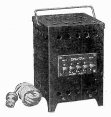
Trade Name-"Spartan"; Type-Bulb; operates from 110 volts, A.C.; Charging Rate-3 amperes, 4, 6 or 12 volts; charges "B" battery; Material of Case-Iron, blue enameled; Dim.-6 x 6 x 9 inches high; Weight-10 lbs.; Price-\$19.50.
