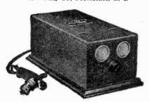
Trade Name—"Rectodyne"; Type—Bulb rec-tifier with filter circuit; uses two tubes (type 201A) to rectify both sides of wave; replaces "B" battery; operates from 110 volts, A.C.; Dim.-6<sup>1</sup>/<sub>4</sub> x 12 x 5 in. high; Price—\$44.00, less tubes. Also made in resistance type with filter eircuit; operates from D.C.; replaces "B" bat-tery; Price—\$32.50.
