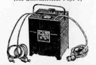
Trade Name—"Balkite"; Type—Electrolytic; operates from 110-120 volts A.C., 60 cycle; also made for 50 cycle; Charging Rate— $2^{3}/_{2}$  to 8 amperes, 6 volts; Material of Case—Terne plate, enameled; Dim.—6 x  $6^{3}/_{2}$  x 9 inches high; Weight—14 lbs.; Price—\$19.50.
