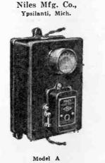
Trade Name—"Niles"; Type—Vibrator; operates on 110 volts, A.C., 60 cycles; Charging Rate—10 amperes, 6 volts; Material of Case— Steel stamping, black crystallized lacquer; Dim. —8½ x 8 x 5 inches high; Weight—14 lbs.; Price—\$19.00.
