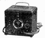
Model 19. Trade Name—"Sterling"; Type—Vibrator; operates from 110 volts, 25, 50 or 60 cycles, A.C.; Charging Rate—5 amperes, 6 volts, with "B" battery connection up to 72 volts; Equipment—Ammeter; Material of Case—Steel; Dim.— $6\frac{1}{2} \ge 7\frac{1}{4} \ge 6\frac{1}{2}$  inches high; Weight— 10 lbs.; Price—For 50 or 60 cycles, \$22.50; for 25 cycles, \$25.00.
