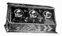
Type-Tuned Radio Frequency; Tubes-6; Bat-tery-"A" Storage or Dry; "B" 135 Volts; Controls-Tuning, 3; Tube, 2; Dim.-7 x 18 x 10; Wt.-21 lbs.
