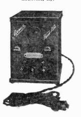
Trade Name-"Power Bee"; Type-Bulb; Oper-Trade Name – Fow face ; Type-Bulls; Oper-ates from 105-120 volts, 60 cycles, A.C.; replaces "B" Battery; delivers current at 0 to 45 volts for detector, and 0 to 130 volts for amplifiers; Material of Case-Metal, enameled; Dim.-4½ x 8 x 7½ in. high; Price-\$27.50.
