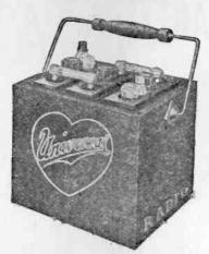
Model No. WR Trade Name — "Universal"; Type — "A"; Capacity—60 A.H.; Material of Case—Wood; equipped with red colored position terminal and bail handle; Finish—Black; Dim.—9 x 7½ x 9%; Wt.—31 lbs.; Price—\$16.00.
