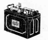
Trade Name—"Cincinnati"; Type—"A"; Capacity—Made in 3 sizes; 70-80, 90-110, 120-140 A. H.; Material of Case—Rubber Composition; equipped with removable handle, screw type lugs; Finish — Black; Dim. — —; Price — \$18.00, \$22.50 and \$28.50.
