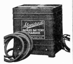
Trade Name—"Standard Duplex"; Type— Bulb; operates from 110 to 220 volts, 25 to 90 cycles, A.C.; Charging Rate—3 to 6 amperes, 6 to 12 volts; 35 to 250 milliamperes, 12 to 48 volts; Material of Case—Sheet metal, enameled; Dim.—7 x 8 x 8 inches high; Weight—18 bs.; Price—Without bulb, \$18.00 to \$22.00. Sterling Mfg. Co., 2831 Prospect Ave., Cleveland, Ohio.
