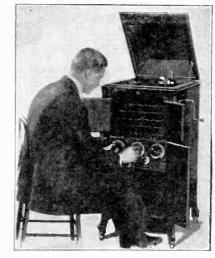
The panel is drawn slightly forward when in use and when not in use is pushed back entirely within the cabinet so that all doors can be closed tightly. This set can be installed in either upright or console models.
