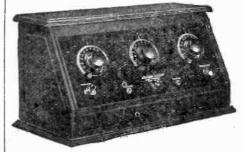
Type — Tuned Radio Frequency; Tubes — 5; Battery—"A" Storage; "B" 90 Volts; Controls — Tuning, 3; Tube, 1; Antenna—None; Price— \$125.00 without accessories.
