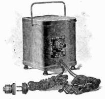
It employs bulb rectifiers, has a safety fuse, color-identified cords, clips for battery terminals, two-piece plug and six feet of cord. It is housed in metal case finished in green enamel.
